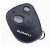
Remote keyless entry (RKE) systems allow a user to lock and unlock the car using a transmitter on the keychain, which transmits data to a receiver in the vehicle. Some of these systems even allow you to start you car by pushing a button. Each car has a unique identification number that is sent from transmitter to the receiver inside the car. In other words, your transmitter will not unlock the doors of your friend's car. Only yours.
